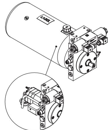
The W83BT series power pack is designed for applications that need high pressure and larger flow, but use a customer supplied low-power transmission. The power pack uses a special manifold (W800553). All screw-in cartridge valves have been designed to be adjusted easily to service the power pack quickly. They still have the same dimensions and functions as the standard manifold (W800532)
